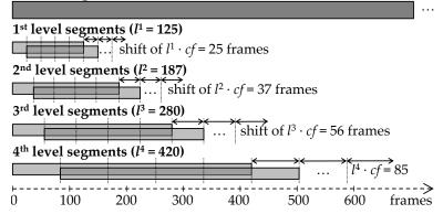
Figure 2.5: Four-level segmentation structure built over a single skeleton sequence [48]. This structure is sufficiently dense to evaluate any query whose length is bounded from 100 to 500 frames (i.e., query duration between 0.8–4.2 seconds in case of the 120 FPS rate). The *i*-th level contains segments of the same length  $l^i$  that are shifted by  $cf \cdot l^i$  frames, where cf = 0.2 stands for the segmentation density factor.
