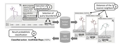
Figure 2.4: Schematic screenshot of the action-recognition application [42]. The input motion is selected as a subsequence between 740–840 frames (i.e., roughly between sixth and seventh second) and finally recognized as the "kickRSide1Reps" class with the 100 % probability, since all the three most similar retrieved actions correspond to that class.
