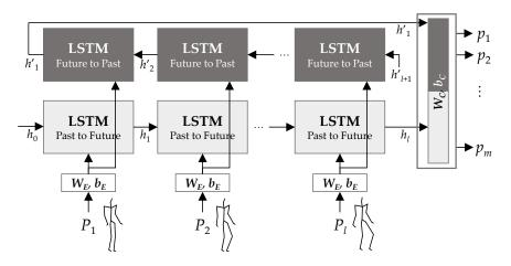
Figure 2.2: Schema of the Bi-LSTM architecture trained on the classification task [44] – individual action poses  $P_1, \ldots, P_l$  are gradually embedded into LSTM cells in both past-to-future and future-to-past directions to determine classification probabilities  $p_1, \ldots, p_m$  of *m* classes. The action feature can then be extracted by concatenating the hidden states  $h'_1$  and  $h_l$ .
