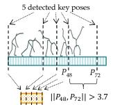
(c) Key pose augmentation: five key poses are detected, where the distance between any two consecutive key poses is higher than the key pose threshold set to 3.7.
