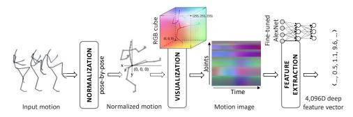
Figure 2.1: Illustration of the CNN feature extraction process outputting the fixed-size 4,096D vector for the input motion of a variable length.
