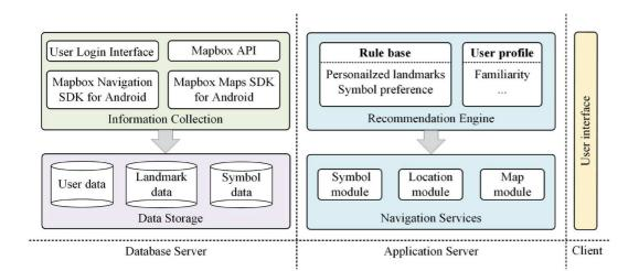
FIGURE 7 Prototype system architecture
