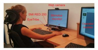
FIGURE 4: Laboratory setting for EyeTribe and SMI accuracy comparison.
