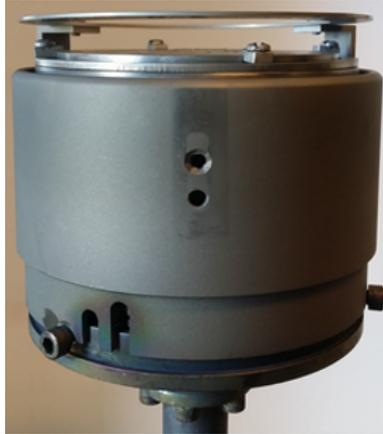
**Figure 2.3:** Magnetron head configuration with custom-made anode.
