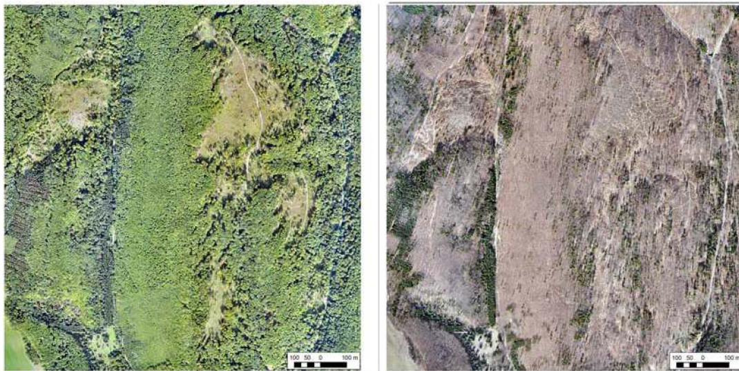
FIGURE 4.14 Orthomosaics from leaf-on (left) and leaf-off season (right) created from images acquired by a fixed-wing UAS.
