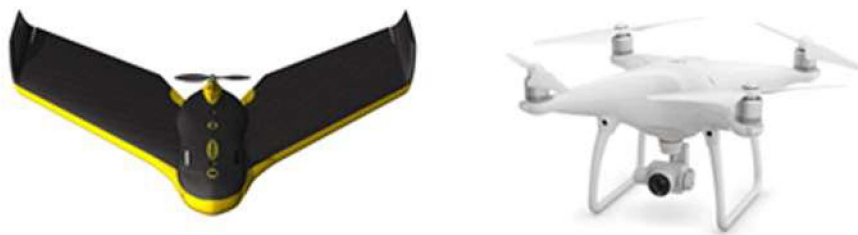
FIGURE 4.6 UASs used for detecting seagrass. Left, a fixed wing EBEE X RTK, right, a Phantom 4.
