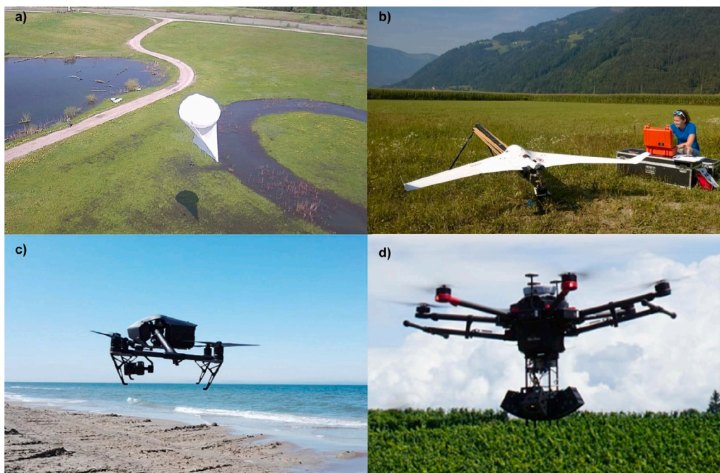
Fig. 1. Different platforms and sensors in UAS surveys; a) Lighter-Than-Air Helikite Balloon with Sony A7RII used for renaturation monitoring; b) BRAMOR ppk Fixed-Wing with Micasense Red Edge used for riparian vegetation monitoring; c) DJI Inspire 2 with zenu-muse x5s RGB camera, used for shallow water vegetation and beach cast monitoring (Palanga, Lithuania), and d) Leica Aibot AX 20 with multidirectional sensor prototype (5 Sony ILCE-QX1 RGB sensors for capturing NADIR and 4 oblique images). (For interpretation of the references to colour in this figure legend, the reader is referred to the web version of this article.)
