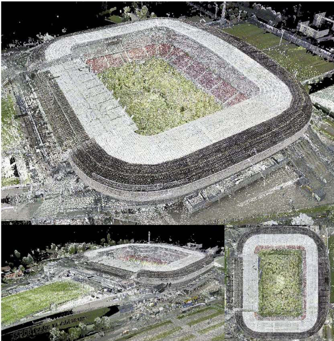
FIGURE 4.11 Integrated UAS – TLS 3D colored point cloud (27,419,265,887 points).
