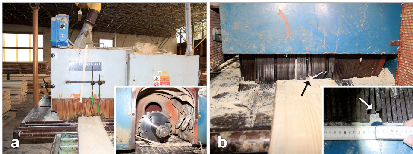
FIG. 1—Circular rip saws consist of a roller conveyor, a feeder with metal kickback slats, and different number of blades (a). Injuries suffered by rip saw operators resulting from mechanical deformation and loss of metal kickback slats, followed by an ejection of a wood splinter (arrows in b). [Color figure can be viewed at wileyonlinelibrary.com ]
